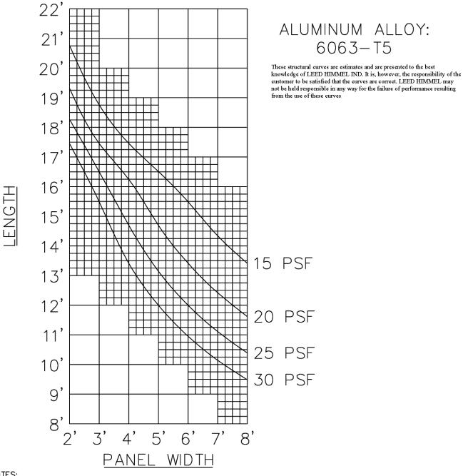
NOTES: - THESE WIND LOAD CHARTS ARE BASED UPON THE LESSER OF DEFLECTION (L/175 OR 1" MAXIMUM) AND STRESSES IN THE ALUMINUM. - THE ALLOWABLE STRÉSSES IN THE ALUMINUM IS BASED ON A MAXIMUM UNBRACED LENGTH OF 16'-0", UNBRACED LENGTH GREATER THAN 16'-0" REQUIRES ADDITIONAL ENGINEERING.
