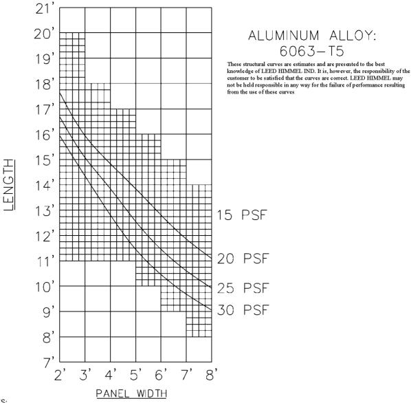
NOTES: - THESE WIND LOAD CHARTS ARE BASED UPON THE LESSER OF DEFLECTION (L/175 OR 1" MAXIMUM) AND STRESSES IN THE ALUMINUM. - THE ALLOWABLE STRÉSSES IN THE ALUMINUM IS BASED ON A MAXIMUM UNBRACED LENGTH OF 6'-0", UNBRACED LENGTH GREATER THAN 6'-0" REQUIRES ADDITIONAL ENGINEERING.
